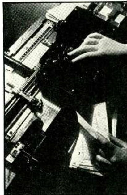
Automatic indexing and sorting machines were used to tabulate the millions of letters in the NBC mail survey
