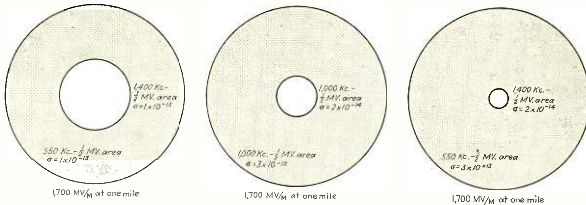
Figs. 1—3. Coverage areas, showing the effects of frequency and soil constants, all referred to a field strength of 1700 MV/M at one mile. The shaded areas show the increased coverage made possible by low frequency assignment, high soil conductivity, and by the combination of the two factors
