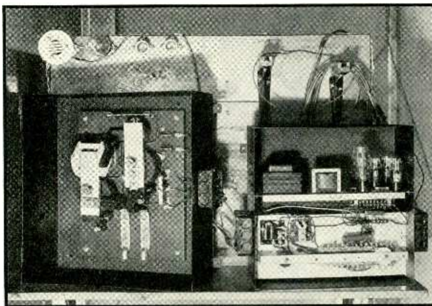
Welding timer "on location"
