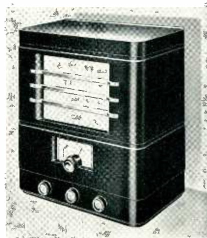
English radio set with Bakelite Molded cabinet. Size: 17" x 14" x 9".
